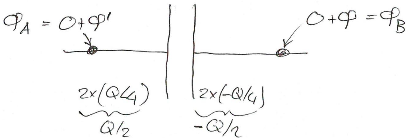
In the superposition, charge  $+Q$  ④ is placed on node A, and charge  $-Q$  is placed on node B, as asked in the problem.
