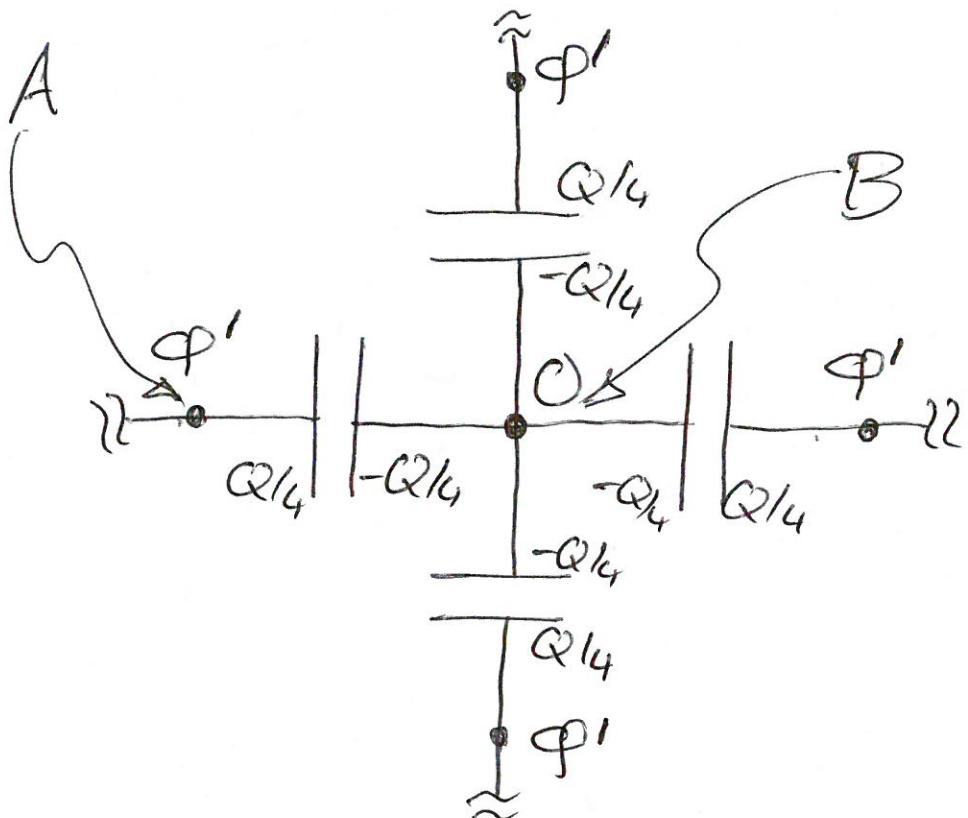
$\phi' = \frac{+Q/4}{C}$ . Now superpose the two drawings, focusing on nodes A, B and the charge on the capacitor between them:
