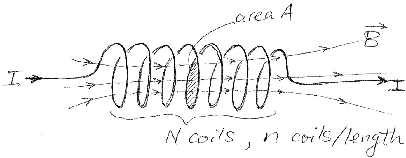
The magnetic field generated by the current is very uniform within the solenoid and decays rapidly with distance on the outside (like a dipole),
