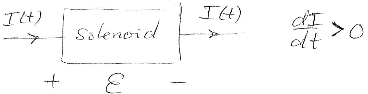
The net EMF  $\mathcal{E}$  is the sum of EMFs around all  $N$  coils, or equivalently, that associated with changing flux through the combined area  $N \cdot A$ :
