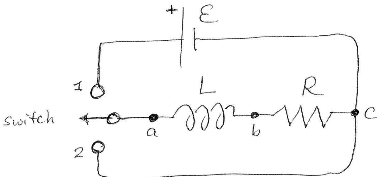
We start with the switch in the ① position. Previously, ignoring the effects of inductance (inductor = idealized wire) we would have ~~concluded~~ concluded the current jumps instantaneously to the value  $\mathcal{E}/R$  in the upper loop when the switch is closed. To see what actually happens we ~~can~~ apply Kirchhoff's
