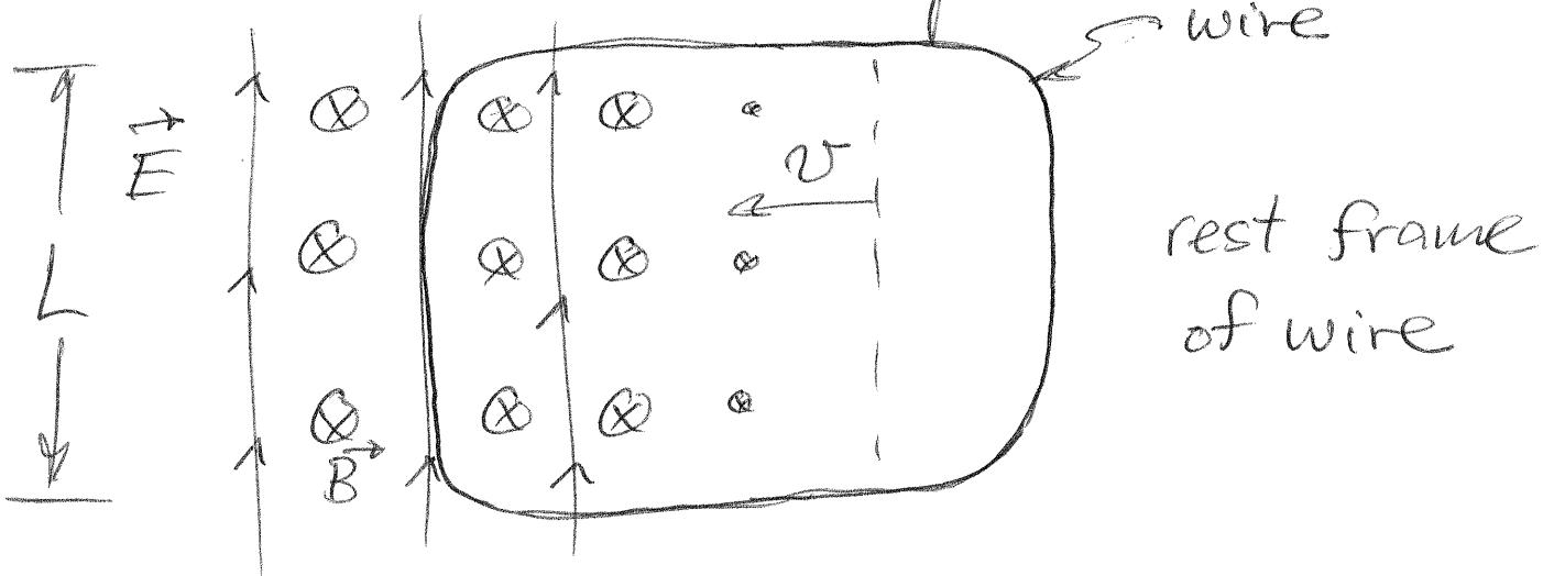
In the rest frame of the wire ③ there is an electric field  $\vec{E} = -\vec{v} \times \vec{B}$  (upward in drawing).
