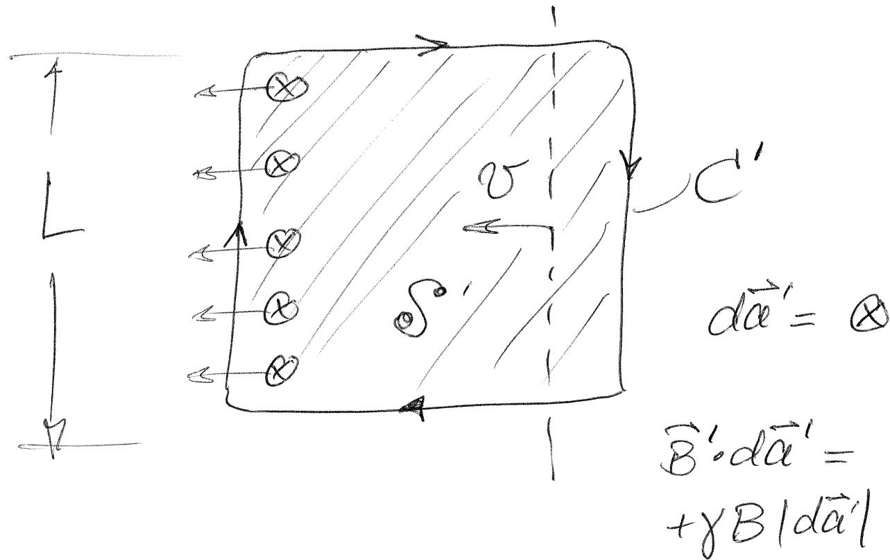
$$\frac{\Delta \Phi_B}{\Delta t'} = - \frac{\gamma B L (0 - \Delta t')}{\Delta t'} = - \gamma B v \Delta L$$
