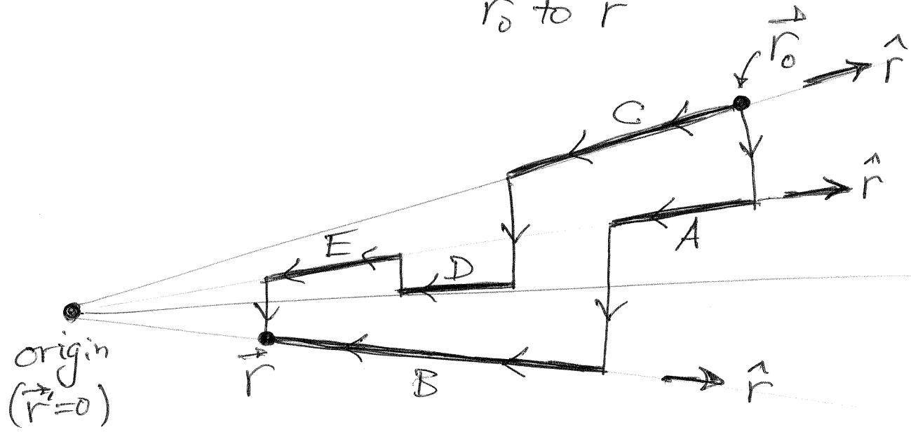
$\vec{F}_{21}$  is (anti)parallel to  $d\vec{r}'$  on pieces A, B, C, D, E and perpendicular on the other parts. Only the radial pieces (A, B, C, D, E) contribute to the line integral. And since  $\vec{F}_{21}(\vec{r}')$  depends only on  $|\vec{r}'|$
