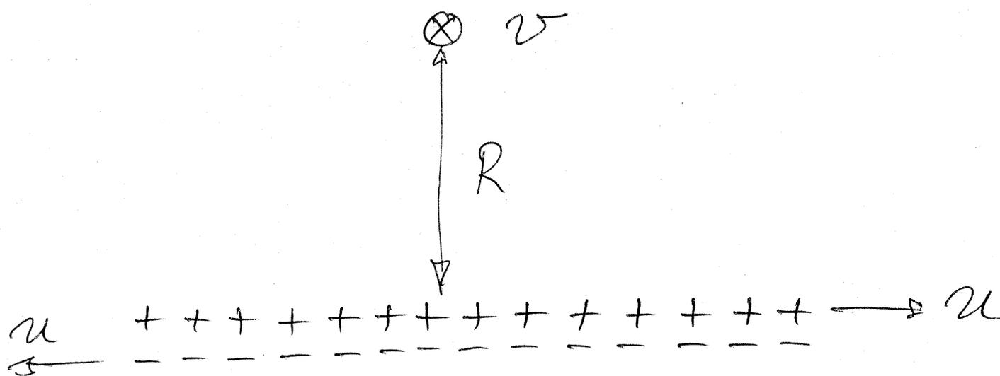
The ~~•~~ ⊗ symbol indicates the test charge velocity is into the page. Like the first case, here the relative motion between line charges and test charge is perpendicular to the electric field. However, unlike the first case the relative speeds for the + line and - line are the same, giving equal enhancement factors. The two fields  $\uparrow E_0\gamma$  and  $\downarrow E_0\gamma$  will therefore cancel.
