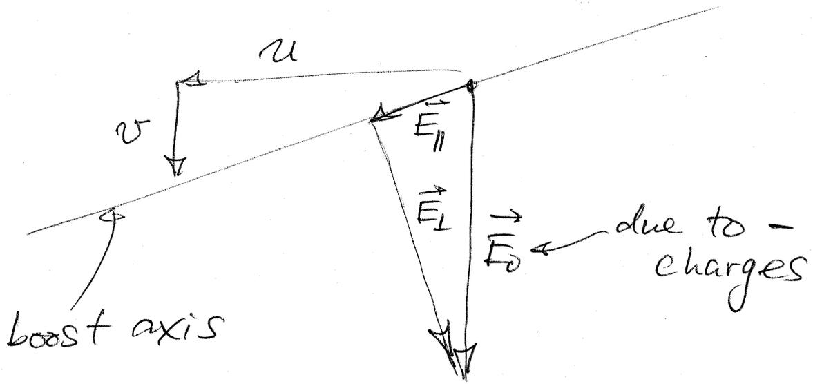
Here's a diagram that combines both fields, showing the enhancement of the perpendicular components:
