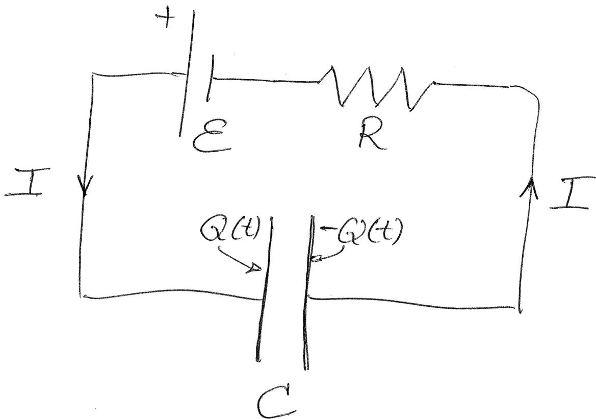
We have seen the pure emf and resistor before (the latter would be the internal battery resistance). The new circuit icon, a pair of parallel lines (plates), represents the capacitor. Because there is no net charge flowing into the battery (note current arrows), there is also no net charge flowing into the capacitor. However, there is net charge  $\pm Q(t)$  accumulating on the two capacitor plates. Working out the function  $Q(t)$  will be our next task.
