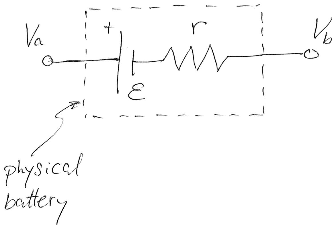
The potential  $V_a - V_b$  across the terminals of the battery now also depends on the amount of current  $I$  flowing through the
