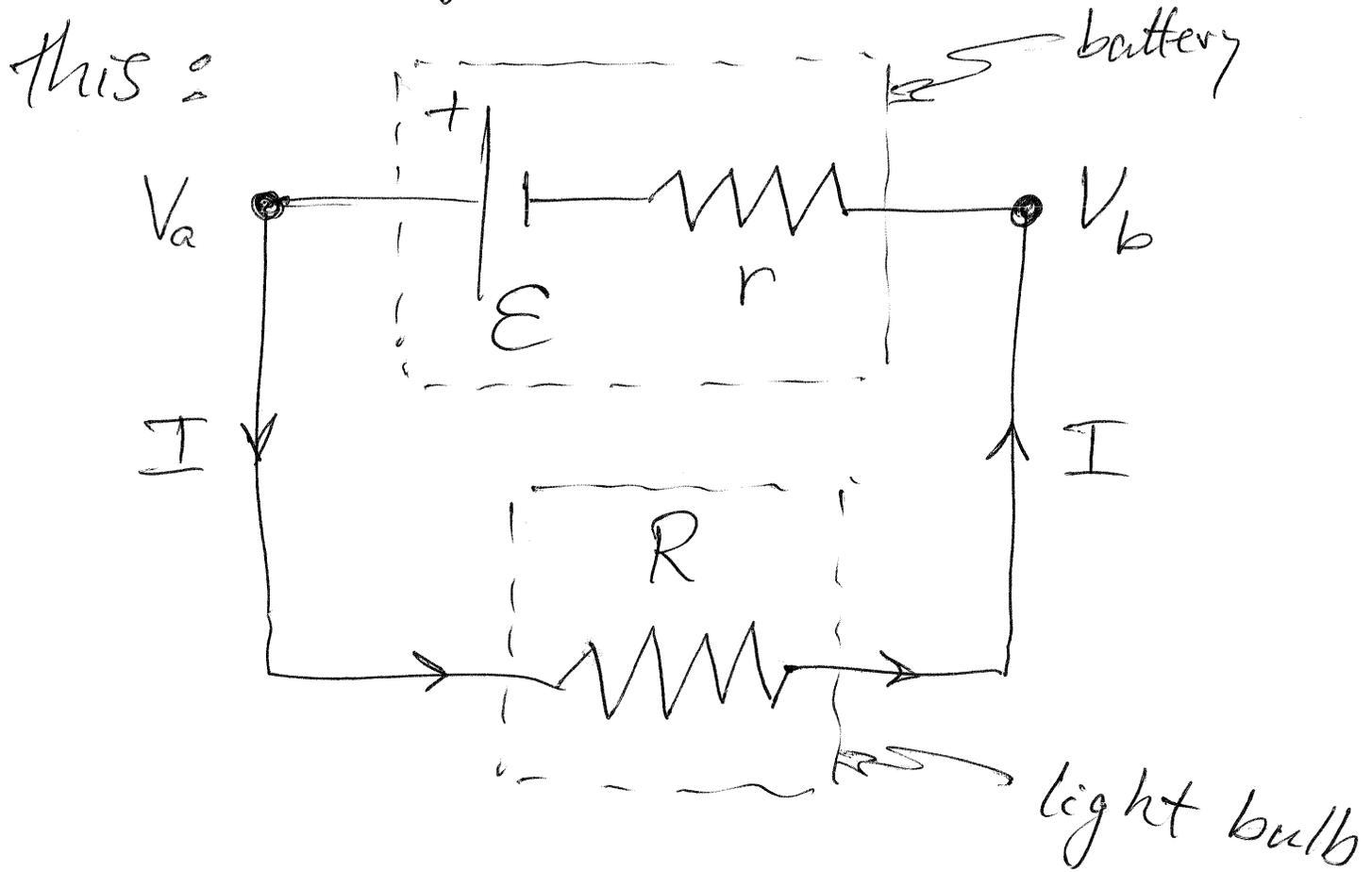
The light bulb is represented <sup>(4)</sup> as a resistor  $R$ , since its action on the flow of charge is no different. In a light bulb the electrical energy is dissipated in a very small amount of material — a thin filament — so that it becomes very hot and emits radiation (electromagnetic waves, actually!). The strong temperature variation of light bulbs has the effect that  $R$  is not as constant as it is in proper resistors.
