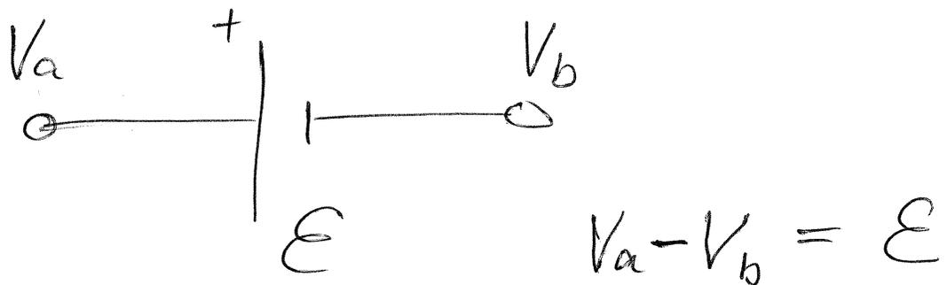
where  $\mathcal{E}$  is the energy per unit charge ~~acquired~~ acquired by charges as they move from terminal  $b$  to terminal  $a$  (the side indicated by "+"). An actual battery will also have internal resistance in addition to the pure emf
