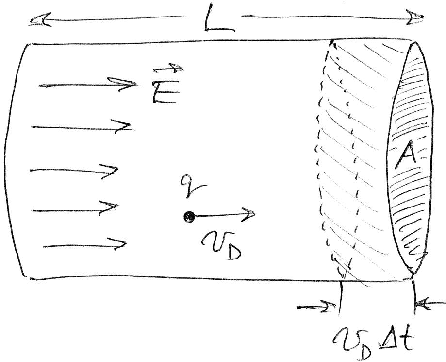
$n$  = number density of charges  $q$  within the conductor
