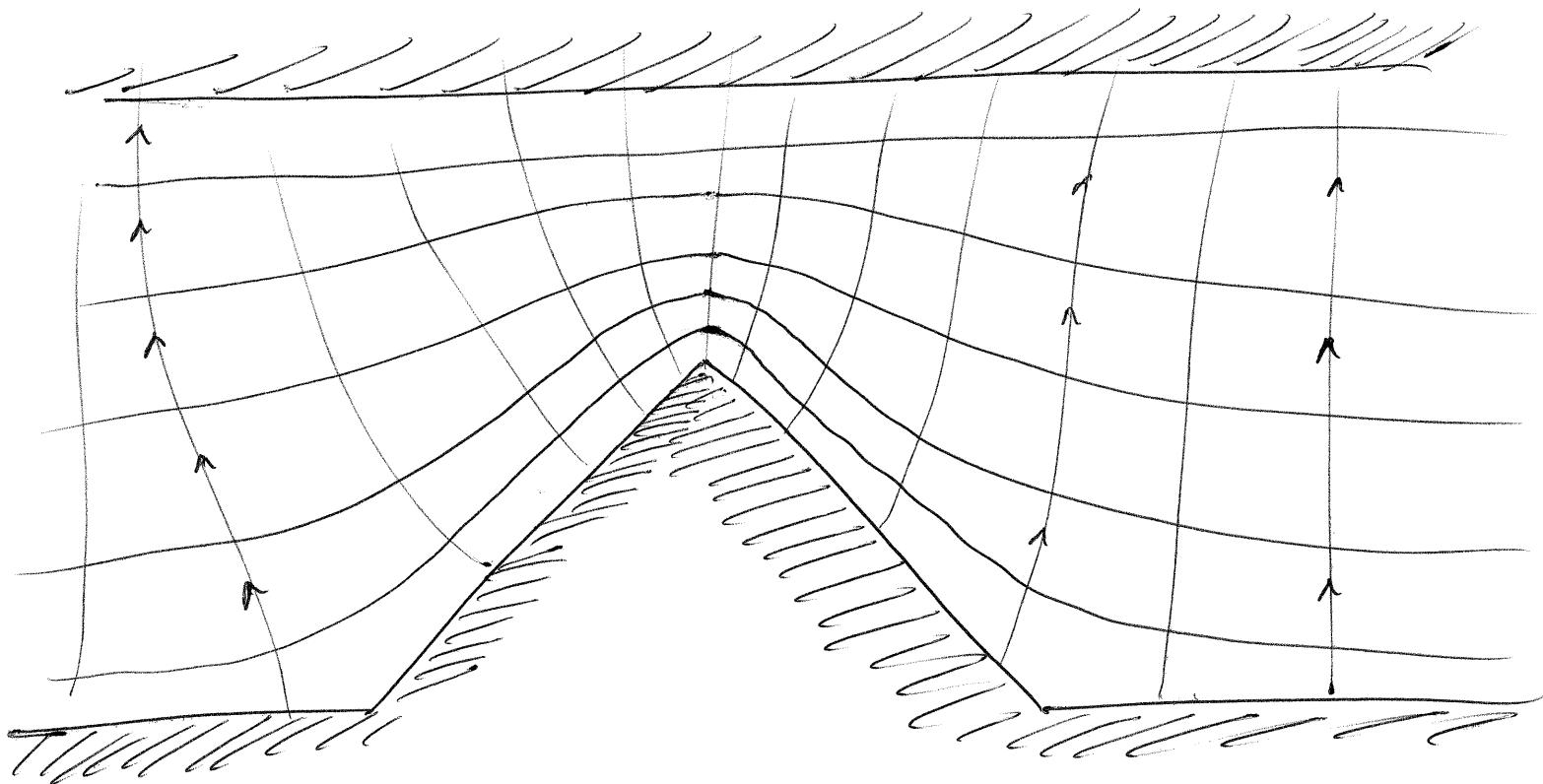
The  $\Phi = \text{const.}$  contours are more compressed around the wedge — they have no choice — and the electric field therefore has a
