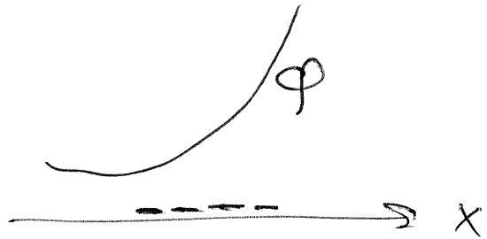
When  $\rho = 0$ ,  $\phi$  doesn't "curve" at all. What exactly does this mean? This is an important special case, one that deserves careful study. It applies, for example, to situations where we have some ~~the~~ conductors in a space that is free of charges. Outside the conductors we have  $\rho = 0$  and therefore
