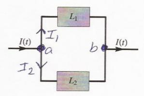
(10 points) The diagram above shows two inductors L<sub>1</sub> and L<sub>2</sub> in a parallel arrangement. Starting from the voltage rule of inductors,
