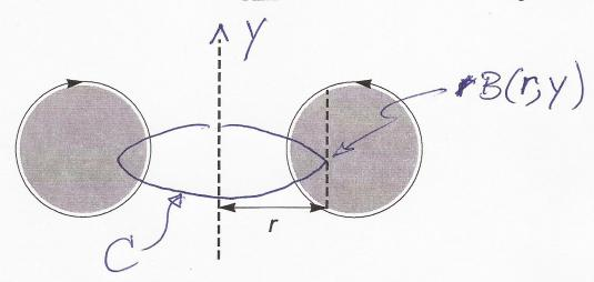
(b) Use the integral form of Ampère's law to argue that the magnitude B of the magnetic field is constant along the dashed line on the right that has a fixed distance r from the axis. Be sure to specify the curve  $\mathcal C$  in your application of Ampère's law.
