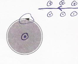
One can show (you are not asked to do this) that the magnetic field B generated by this particular surface current density is purely azimuthal and non-zero only in the interior of the bagel. In other words, B can only point into or out-of the page and is nonzero only in the gray regions.
