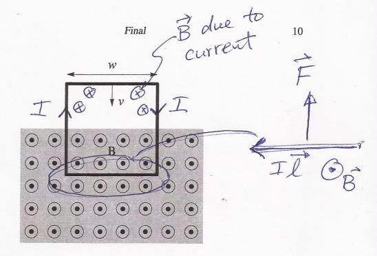
4.  $(15 \ points)$  The drawing above shows a square copper loop moving downward with speed v into the magnetic field of a strong magnet. Assume the field is zero outside the shaded region and uniform of magnitude B and out-of-the-page within the shaded region. The loop has side w and resistance R.
