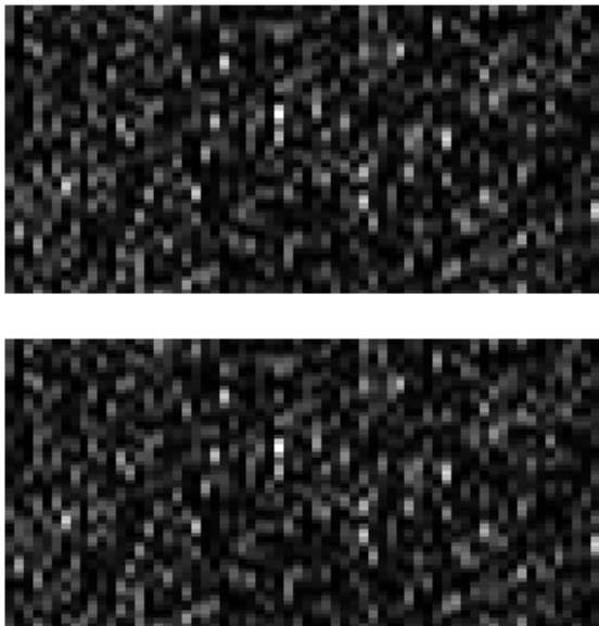
FIG. 1: Top: A diffraction signal comprising 64 continuous one dimensional signals arranged side-by-side. The tomography angle \theta varies vertically. Bottom: Reconstruction of the top signal from 10^4 tomographic measurements (horizontal sections) of unknown \theta . Each measurement was a 64-tuple of photon counts with mean count \mu = 0.32 .
