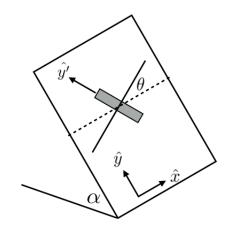
(a) Consider the axis through the wheel that is normal to the plane. Since the length of lever arms of all forces (gravity, normal force and static friction) about the axis equals to zero, the net torque goes to zero. Therefore, the angular momentum of the wheel about the axis is conserved, and the angular velocity  $\dot{\theta}$  equals to a constant  $\omega$ . The time dependence of  $\theta(t)$  is subsequently given by
