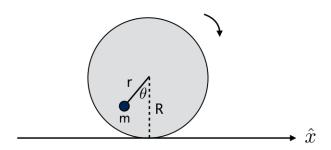
Since the wheel rolls without slipping, the position vector of the mass is given by
