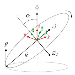
Recall that the total angular velocity  $\vec{\omega}$  of the ring that rolls clockwise without slipping is anti-parallel to the position vector  $\vec{R}$  of the point of contact. Consider the body frame S' with its basis vector  $\hat{\bf 3}$  parallel to the axis of the ring and  $\hat{\bf 1}$  always aligning with  $\vec{\omega}$ . Assume that the ring has linear mass density  $\lambda = M/(2\pi R)$ . The summation of the formula (4.17) in Lecture 4 becomes an integral:
